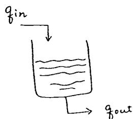
$$\begin{aligned} \text{Volume of tank} &= 100 \text{ gal} \\ \text{Initial Amount of H}_2\text{O} &= 50 \text{ gal} \\ q_{\text{in}} &= 2 \text{ gal/min} \\ k &= 0.1 \text{ min}^{-1} \end{aligned}$$
